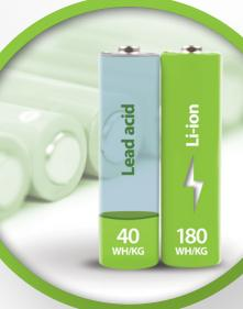
Lithium-ion vs Lead Acid
