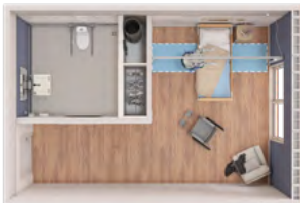
Wall mounted. Linear track with wall posts, for fixed or portable ceiling lifts.
